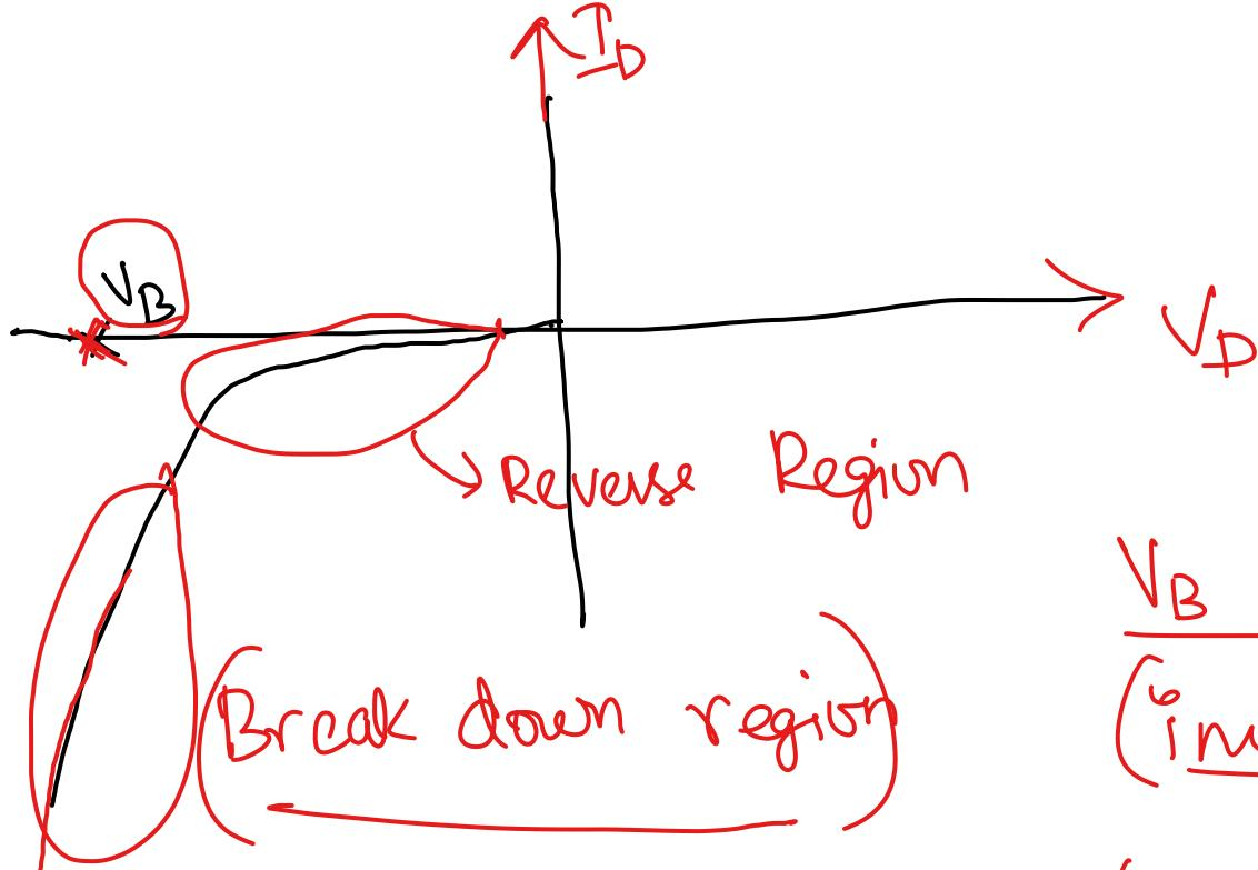
$$\frac{V_B \text{ Break down } V_{tg}}{(\text{impact ionization})}$$
